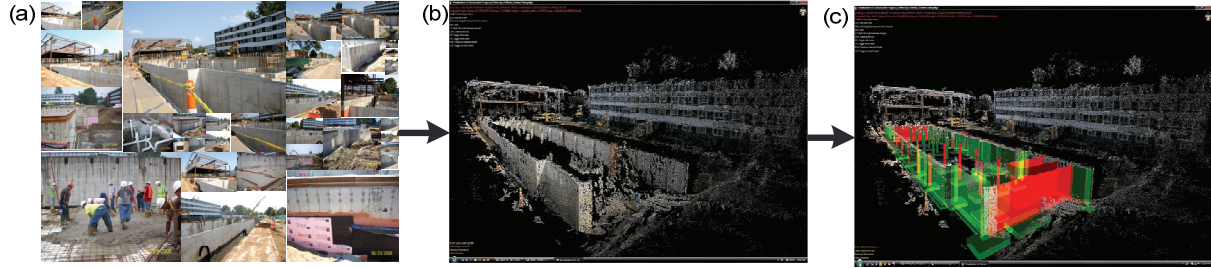
Fig. 2: An overview of the D 4 AR modeling and automated progress monitoring system. (a) Unordered daily construction photographs; (b) Generating 3D/4D as-built point cloud models and registering site images; (c) Generating D 4 AR models by superimposing 4D as-planned Building Information Model with 4D point cloud model and registered images; and automatically detecting physical progress.
